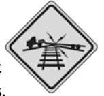
7. **NO TRAIN HORN** sign shall be installed at each highway-rail grade crossing where there is a Federal Railroad Administration authorization for trains to not sound a horn. The sign shall be mounted as a supplemental placard below the Highway-Rail Grade Crossing Advance Warning.
